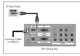
NOTE: Please check if the power of HDMI source is on, in case that you fail to select HDMI from the "Source List" even after you connected the cable of HDMI source (DTV Set-Top Box, DVD, etc.) to TV.
